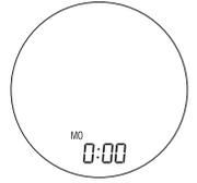
**NOTE:** If you remove the module from its base for more than 6 hours, the time and day must be reprogrammed.
