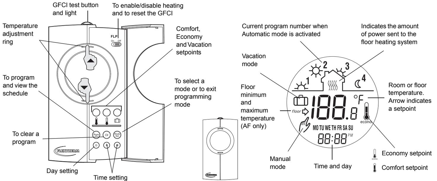
The FLP12-GA programmable thermostat, specially designed for floor heating installations, is equipped with two ultra-precise sensors which allow temperature control by separately monitoring both floor and ambient settings, thus providing greater comfort.
