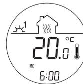
To temporarily bypass the current program, set a new temperature using the adjustment ring or press one of the predefined setpoint buttons (↓ or ↑). The program icon will flash to indicate the bypass. The new setpoint will be maintained until the beginning of the next program.
