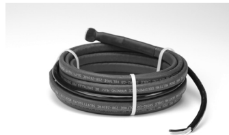
240V cable has an end seal and a cold lead; requires a power connection in an appropriate junction box.
